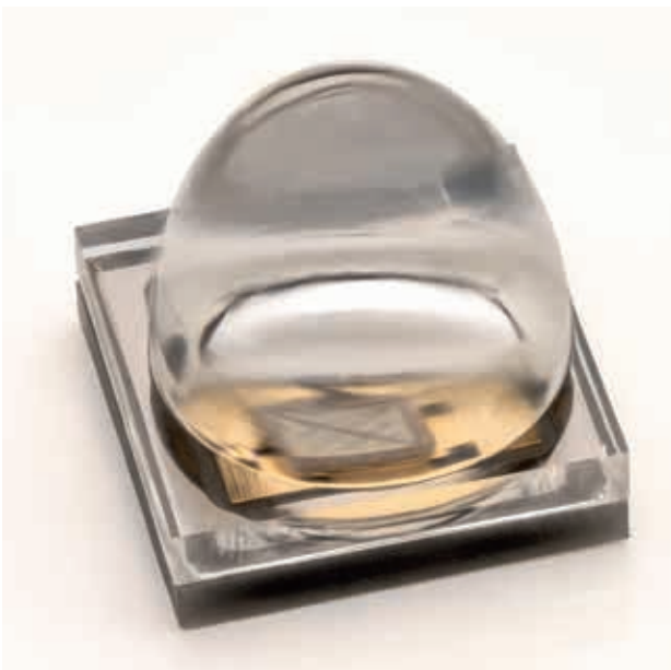
UV LED chip on ceramic submount with quartz lens
